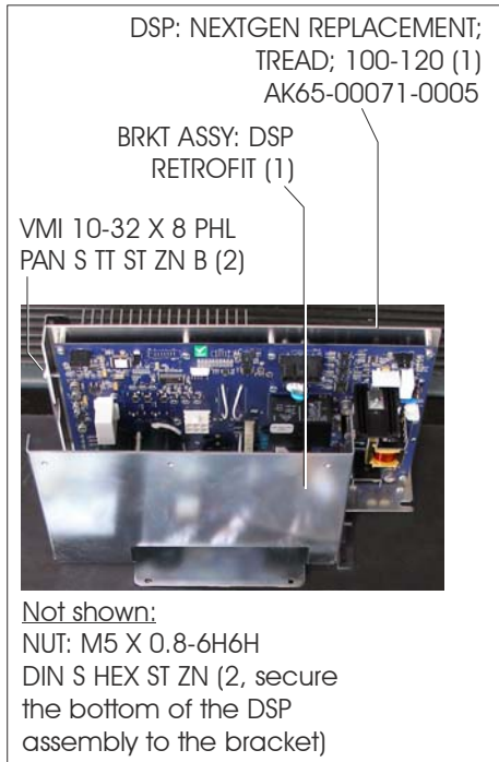
Fig. 1: 120V DSP Retrofit Bracket Assembly
